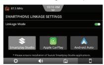
Figure 30: Smartphone Linkage Settings Screen
